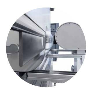
Synchro-Form is a revolutionary new approach to bending large profiles, developed by LVD, an industry leader and innovator. The Synchro-Form system evolves LVD renowned adaptive bending technology to automatically maintain angular consistency and the required geometric profile when bending large parts. Synchro-Form eliminates manual operations, reduces setup and handling, and ensures consistent bending results – delivering high throughput for large bending applications.
